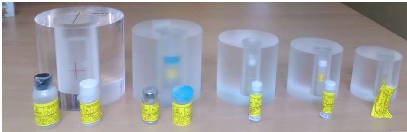
Figure 1 . Thyroid-neck phantoms for adults and children of 15, 10, 5 and 1 years old developed at CIEMAT.
