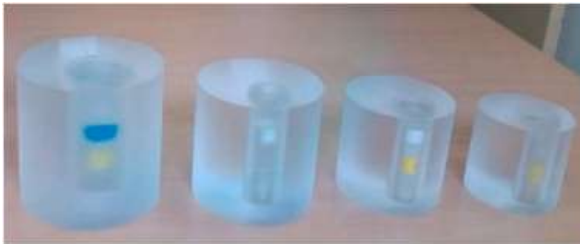
Age-specific pediatric neck and thyroid phantoms (15, 10, 5, and 1-year-old models).
